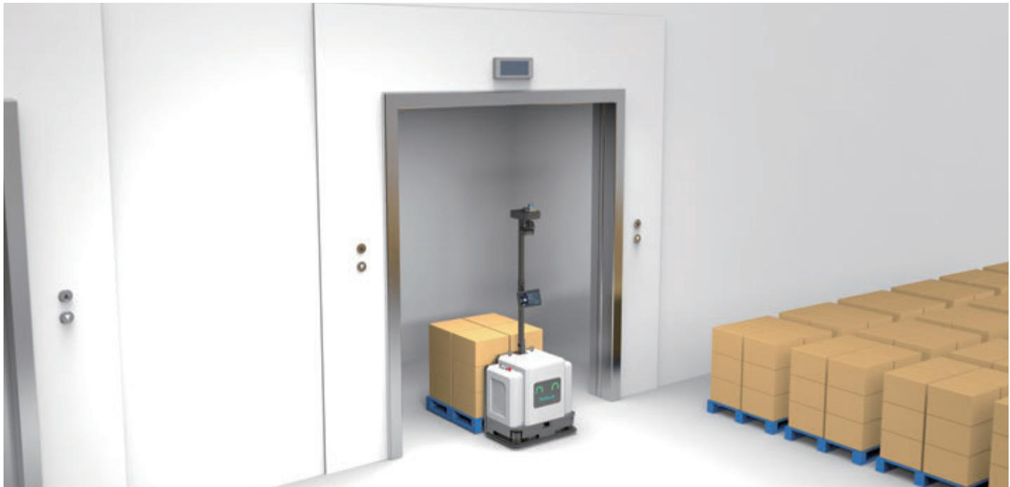
The cross-floor handling function makes it suitable for multi-floor and multi-area material handling applications. With the equipment control system MW-WCS, it can automatically interact with elevators or automatic doors and therefore enter/exit them to walk between different floors and areas.
