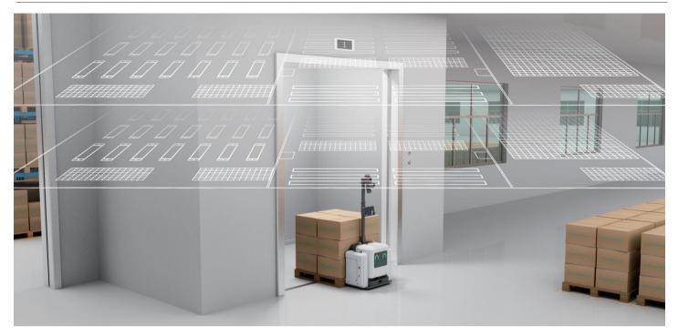
The cross-floor handling function makes it suitable for multi-floor and multi-area material handling applications. With the equipment control system MW-WCS, it can automatically interact with elevators or automatic doors and therefore enter/exit them to walk between different floors and areas.
